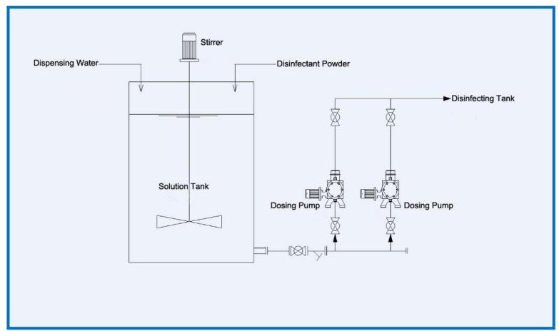
The equipment principle is quite simple, can refit the recent dosing equipment or build a simple dosing system.
